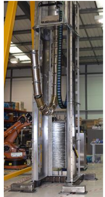
Vertical deployment of LaserSnake2 system
