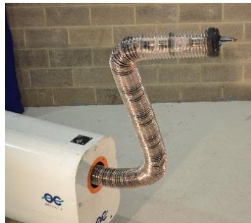
Laser process head integrated with snake-arm robot
