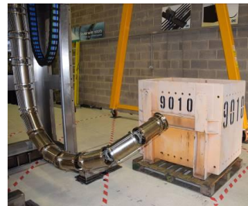
Vertical deployment of LaserSnake2 system
