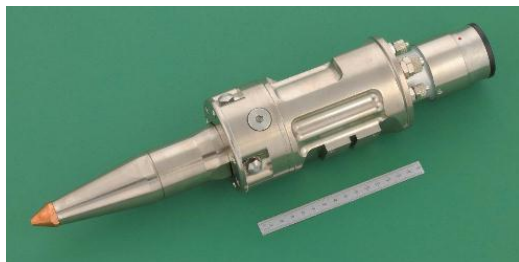
Developed laser process head for LaserSnake2
