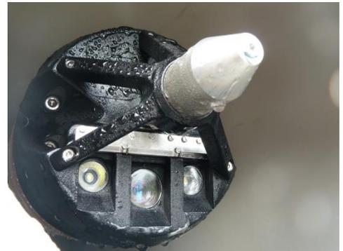
Fig 3. JetSnake tool – water jet, camera and lights
