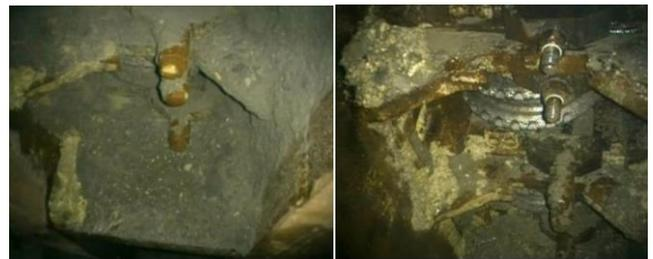
Fig 4. Disc cutter before and after water jet cleaning
