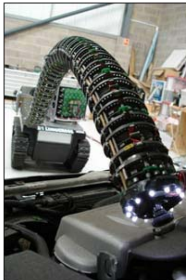
The snake-arm robots have more than 20 degrees of movement
