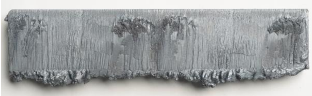
Figure 8. Cut face from a 200mm long sample of C-Mn steel cut using the 250mm lens and the DOE.
