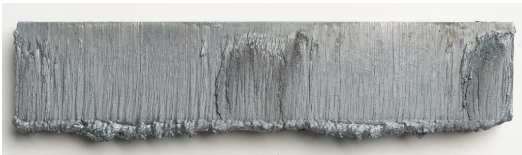
Figure 9. Cut face from a 200mm long sample of C-Mn steel cut using the 500mm lens alone.
