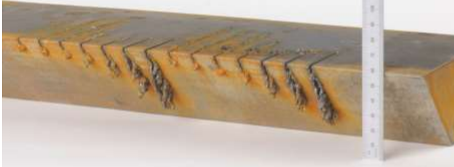
Fig. 2. Series of linear underwater fibre laser cuts across a 45° wedge in a 60mm thickness S355JR+N mild steel block.
