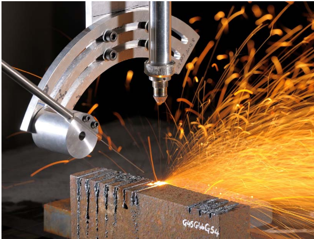
Figure 7 The lower end of the gouge cutting head, showing the conventional co-axial assist gas/beam delivery nozzle and the side gas jet. In this case the side gas is delivered through a narrow stainless steel tube so that, as successive cuts are made, the end of this nozzle can descend into the cutting groove.
