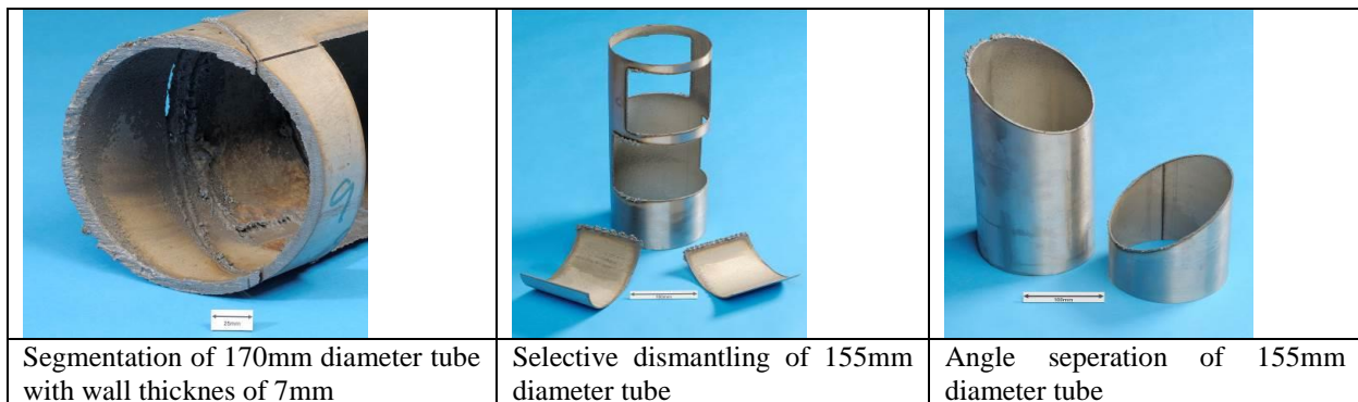
Figure 4. Different cutting strategies allowing removal of sections and cutting at angles not perpendicular to the tube axis.
