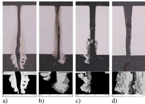
**Figure 8** Cross-sections (top row) of laser cut kerfs produced in 12mm thickness materials using 5kW, at a 15mm focus position, with 8bar cutting gas pressure, at 400mm/min, and associated dross microstructures (bottom row). In each case, the upper image is an optical micrograph and the lower a scanning electron micrograph. In Figure 8d), as dross was not present at the bottom of the kerf, the SEM image shown is that of residual melt inside the kerf itself.
