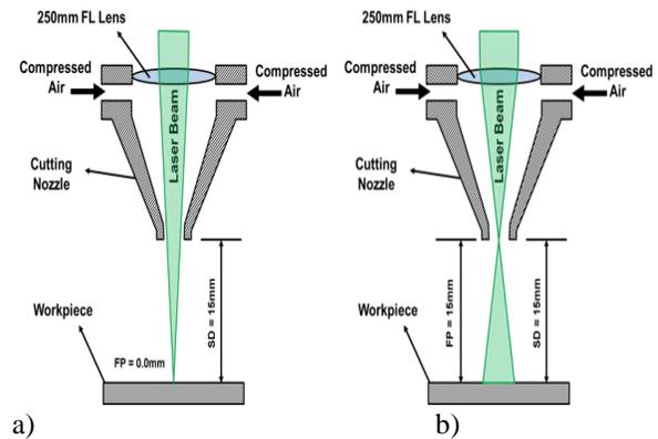
**Figure 2** Laser focus positions with common standoff distance of 15mm used in cutting trials, a) 0 mm, b) 15 mm.
