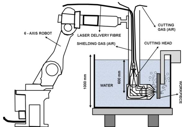
**Figure 1** Schematic of the underwater laser cutting arrangement used
