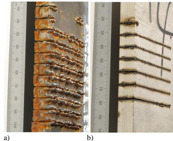
**Figure 3** A view of underwater laser cut kerf exits in 12mm thickness material: a) S275JR C-Mn steel, b) 304 stainless steel
