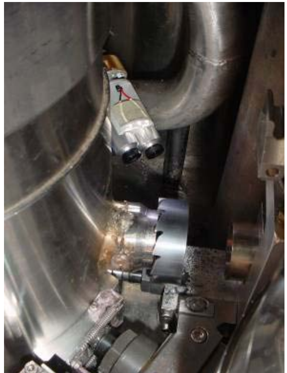
Inspection arm cameras viewing the work site
