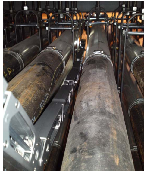
SAFIRE with arm deployed below the walkway (in mock-up)
