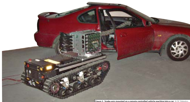
Figure 2. Snake-arm mounted on a remote controlled vehicle reaching into a car © OC Robotics
