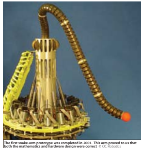
The first snake-arm prototype was completed in 2001. This arm proved to us that both the mathematics and hardware design were correct © OC Robotics
