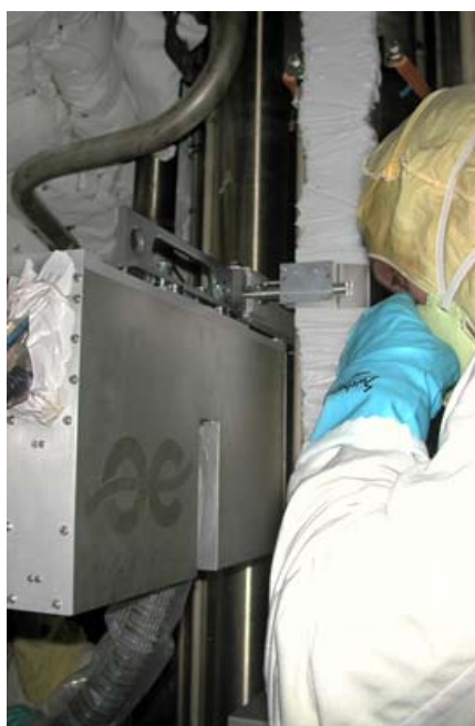
Figure 10: Manipulation Arm fully assembled in the CIR
