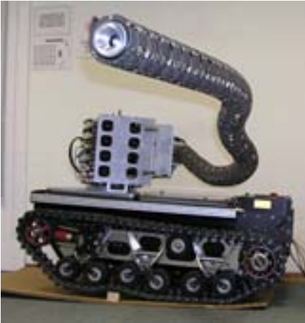
Figure 4 - 2.5m snake-arm robot for UK MoD
