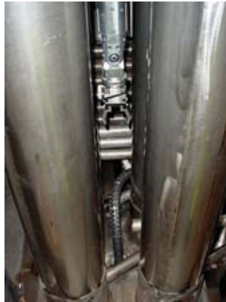
Figure 5 - The Inspection Arm carried cameras to the work site
