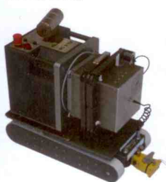
Figure V.4 OPG system: mobile unit with snake-arm stowed coiled
