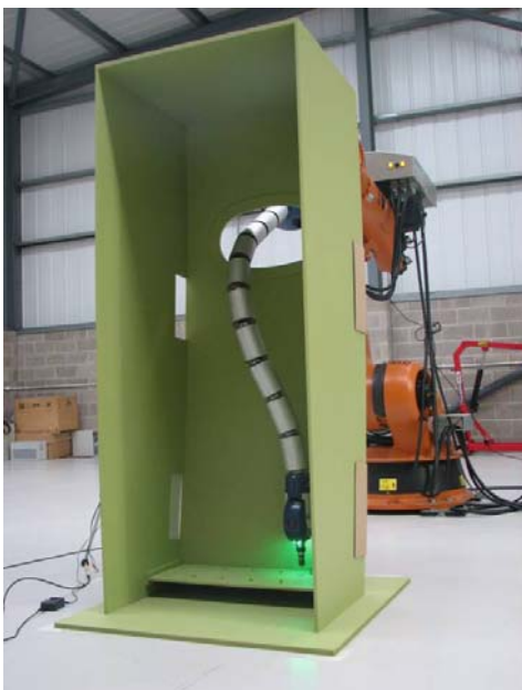
Figure 3 - Snake-arm robot reaching into a rib bay mock-up
