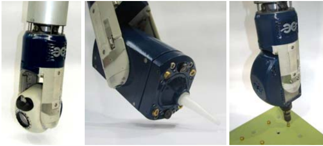
Figure 5 – (Left to right) inspection tool; sealant tool; swage tool
