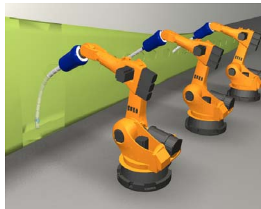
Figure 6 – Snake-arm robots on an assembly line
