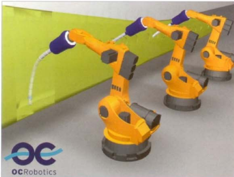
Fig. 2. The prototype snake-arm has the flexibility to enable it to enter the rib bay of a wing-box.
